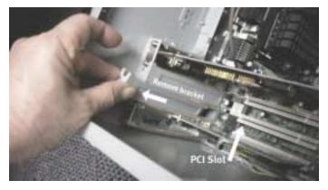
Insert your 3Com ADSL Modem PCI into the slot where you just removed the bracket. Do not touch any of the electronics on the board. Hold the modem from the edge and firmly press it straight down. Do not force the modem into the slot. Make sure it is fully seated in the slot. Then, screw it into place using the screw you removed from the bracket.
